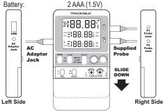
Probe labeled P1 must be plugged into the probe jack labeled "P1" and probe labeled P2 must be plugged into the probe jack labeled "P2".
