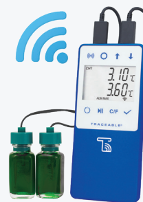
Traceable® Refrigerator/Freezer Data Logger Thermometer
