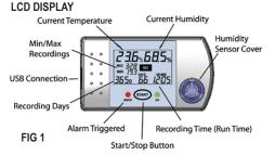
Current Temperature – The current temperature reading Current Humidity – The current humidity reading Min/Max Recordings – The minimum and maximum temperatures that have occurred since the device was initialized.
