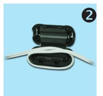
Loop the right end of the cable under the suppressor and back up again laying the cable along the center of the suppressor.
