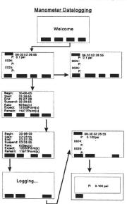
.Before logging, make sure you have set up the parameters by pressing SET key , or you will see a blank data .
