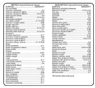
When the emissivity of an object is unknown use a non-infrared thermometer, such as a thermometer with a surface probe to measure the object's surface temperature. Adjust the emissivity until the temperature of the infrared thermometer matches the temperature of the surface probe. The emissivity value arrived at by this method may be used to measure similar materials.
