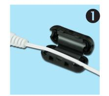
Lay the cable along the center of the suppressor with the connector to your left.
