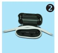
Loop the right end of the cable under the suppressor and back up again laying the cable along the center of the suppressor.
