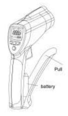
Locate the indentions on either side of the plastic case near the trigger. Open the battery compartment by pulling the rubber portion of the handle out and away from the trigger. *Pull hard, it requires a good amount of force to open the battery compartment.*Remove the exhausted battery and replace it with a new 9-volt alkaline battery. Close the battery cover by snapping it shut.
