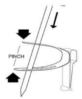
bottom of the holder. When the ends of the holder are released, the holder will expand to grab the probe securely. Use the clip to attach the holder to the side wall of a container. To remove the holder, pinch the ends of the holder and remove the probe.
